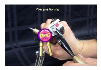
Position pliers so that the top plier is above the <u>Joint</u> and the bottom plier is below the <u>Joint</u>. Apply enough pressure to the <u>Top cap</u> and <u>Base</u> so that the <u>Top cap</u> and <u>Base</u> do not spin in the jaws of the pliers. Hold the bottom pliers still and turn the top pliers counter-clockwise to loosen the <u>Top Cap</u>.
